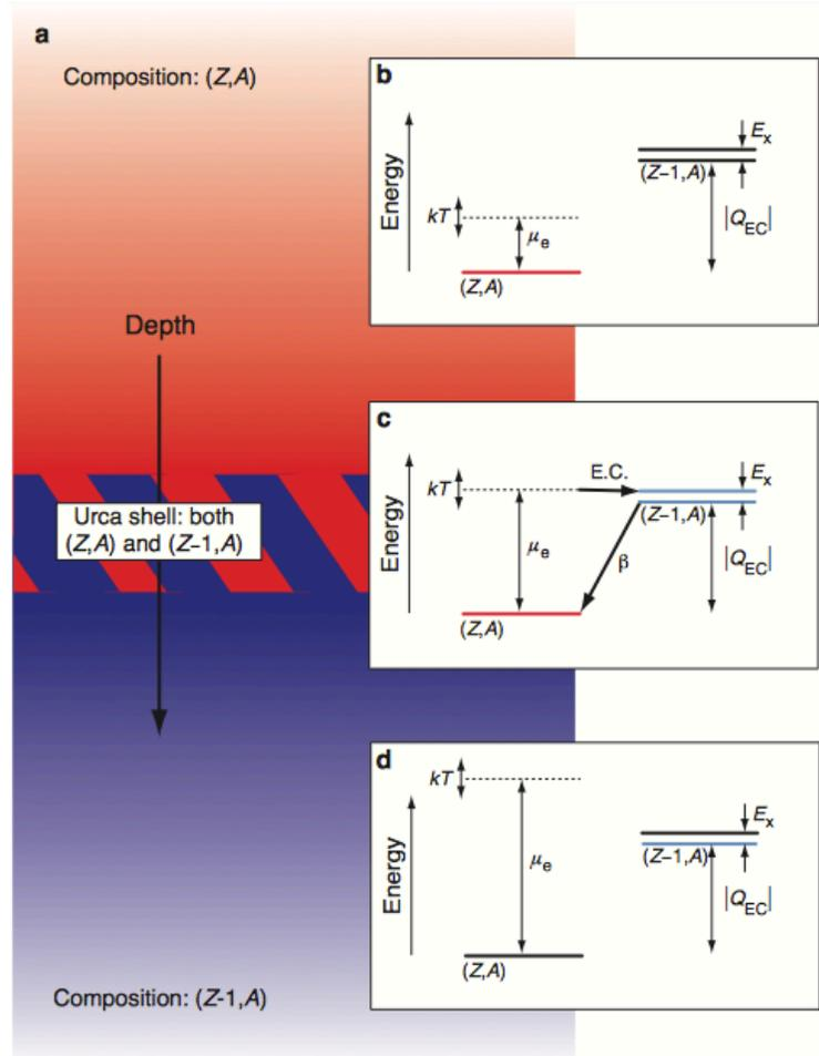
Illustration of compositional layers in the neutron star crust; b–d, energy level diagrams. In the Urca shell between the regions with composition  $(Z,A)$  and  $(Z-1,A)$   $\mu_e \approx |Q_{EC}|$ . As a result, both electron capture and  $\beta^-$  decay are possible, and rapid cycling between the nuclei  $(Z,A)$  and  $(Z-1,A)$  leads to a strong neutrino emissivity.
