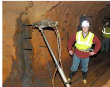
Left: Dr Jose Alonso, Director of Sanford Lab at Homestake, inspects a jackleg drill on the 4550 Level. The jackleg is the iconic tool of hardrock mining. Technicians were using this one to install pins to hold dewatering pipes.
