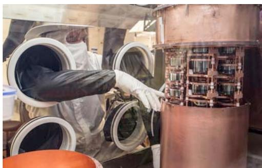
*Figure 4: MAJORANA researcher Matthew Green test fits a copper cryostat loaded with seven strings of germanium detectors*
