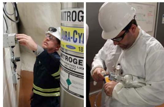
*Figure 6: Left: Facilities Tech Shane Heydon prepares oxygen sensor in the MJD liquid nitrogen alcove for calibration; Right: Dana Byram uses a handheld gas tester to check oxygen concentration of calibration gas*
