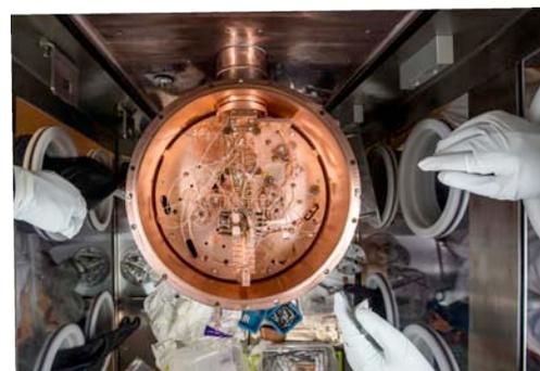
*Figure 4: One of the cryostats used in MJD. The final e-beam weld is on the top side of the image, right before the crossarm tube goes into the big copper plate wall*
