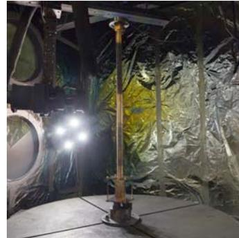
*Figure 3: Cryo 1 thermosyphon tube just after welding at EBWA on January 31, 2014*
