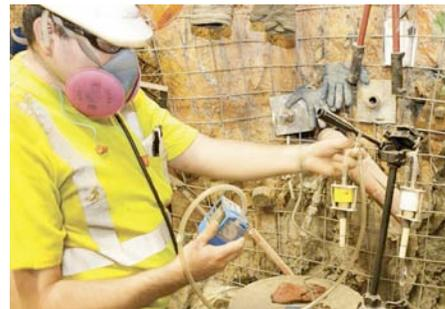
*Figure 9: Industrial hygienist Jason Rosdahl regularly inspects airflow rates on the 4850 Level Davis Campus to ensure that dust and diesel particulate matters (DPM) are within acceptable limits*
