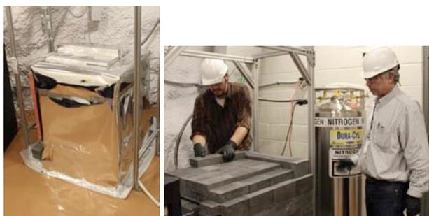
*Figure 3: Left: The final shield around CUBED is a Mylar screen; Right: Vic Gehman and Kevin Lesko place a brick on the reconfigured shield*
