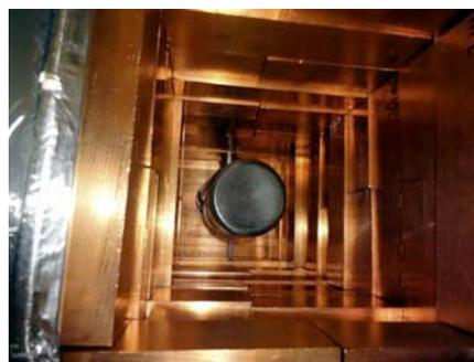
Figure 1: The cavity of the CUBED low-background counting station
