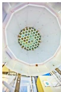
*Figure 4: View beneath the LUX dark matter detector during its construction. LUX uses photo multiplier tubes to detect faint interactions in liquid xenon.*
