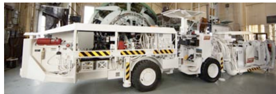
Figure 9: The new rock bolter located in the Yates Hoist room after arriving at Sanford Lab. It will be disassembled, lowered, and then reassembled underground
