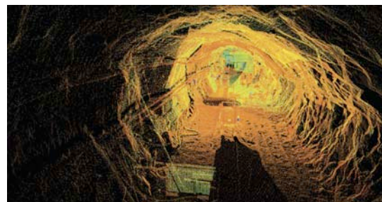
Figure 6: A laser scan creates a digital file called a point cloud. The point cloud can be moved and rotated in 3D space or used in CAD software
