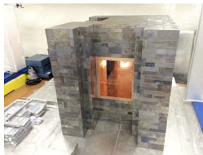
Figure 4: In March, the lead shield of the MAJORANA DEMONSTRATOR was completed. The shield has approximately the weight of a Boeing 737
