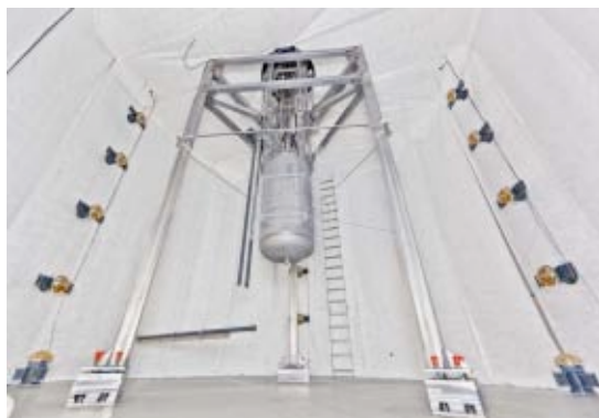
Figure 2: The LUX dark matter detector, inside its water tank
