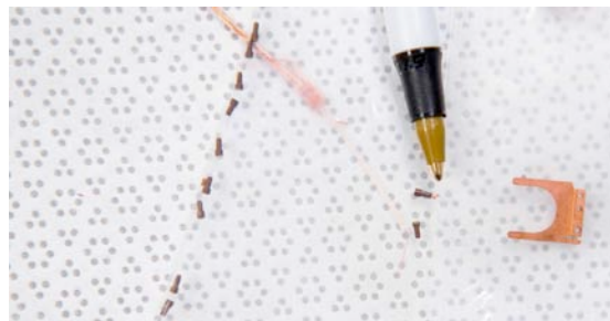
Figure 4: Tiny parts made in the MAJORANA machine shop. These small pins will hold the conductive wire in the copper clip at the right. (Pen is shown for scale.)
