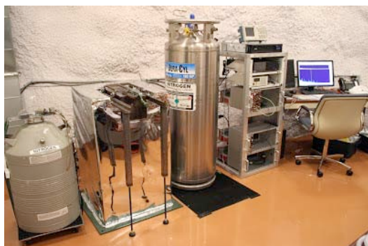
Figure 2: The recently installed BLBF HPGe spectrometer and associated equipment at SURF
