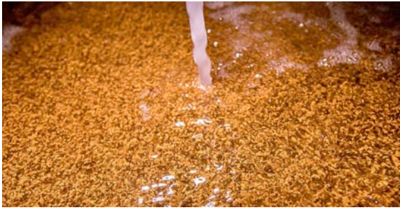
Figure 7: Flocculant is added to the iron-rich water pumped from underground
