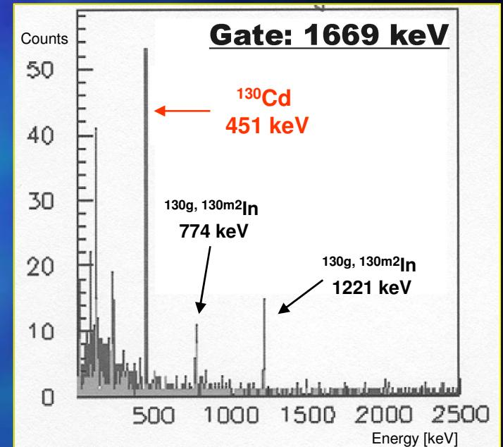
Laser OFF: only surface-ionized elements with low ionization potentials (e.g. Cs, In)
