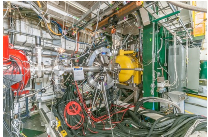
Figure 2. Set-up for (t, ^3\text{He}+\gamma) experiments at the S800 spectrograph with GREINA – a special target transport system was put in place to insert the volatile ^{88}\text{Sr} target (picture credit: S. Noji).
